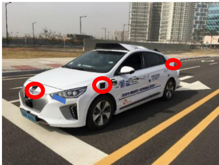
IONIQ (BEV) with 5 pcs of 4D Imaging Radar (LRR, SRR)
