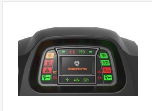
F-Series Excavator MCU 4.3inch LCD
