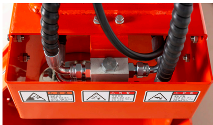
A Case Drain to Protect Hydraulic Motor
