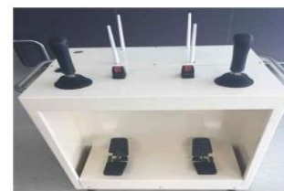
Fig 4. Remote control system of unmanned / remote test equipment
