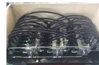
Fig 2. Hydraulic control system of unmanned / remote test equipment
