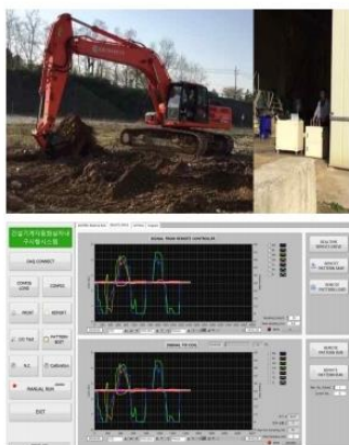
Fig 5. Test results of unmanned / remote test equipment for actual vehicle test of construction equipment
